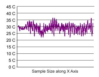
This provides a quick and easy way to analyze and trend host chassis internal temperatures over an extended duration (up to 7+ years). The DDRdrive SuperCap PowerPack is guaranteed maintenance-free for the **entire** 5 year warranty period when temps are less than or equal to 40C.
